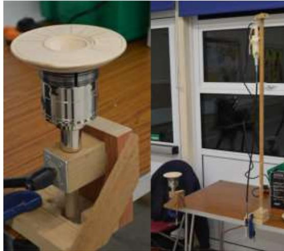
The mount allows the piece to remain in the chuck used for turning so it can be returned to the lathe for any further work.
